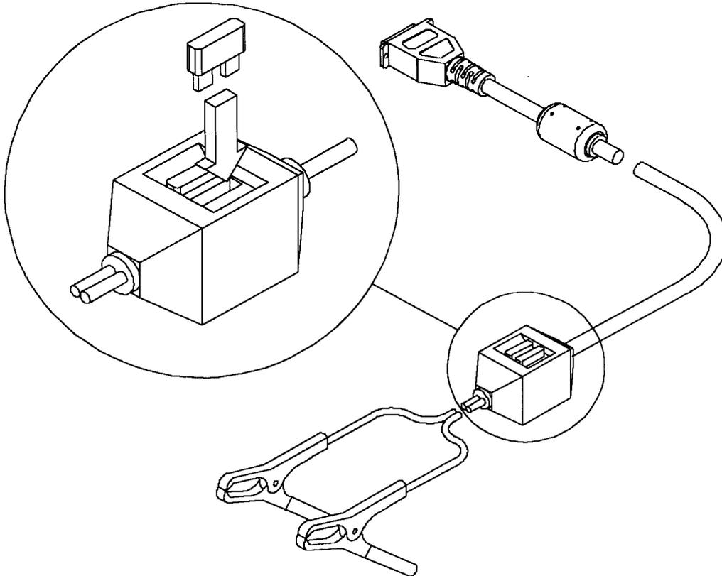
1. Pull 15 amp fuse from battery power cable.
