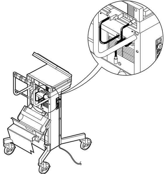
The next stage is to install the portable DeskJet printer into the trolley. Place the printer into the cradle on the trolley. Note that the power and printer interface sockets are positioned on the same side of the trolley as the mains feed cable and switch (i.e. on the right as viewed from the back of the trolley).
