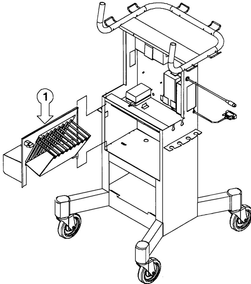
1. Put hinge into securing hole.
