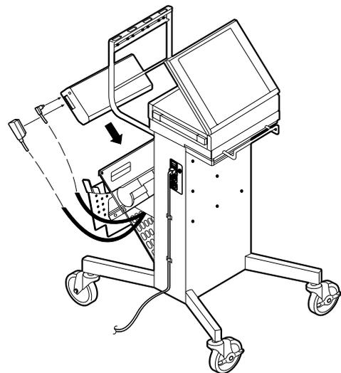
Connect the printer power cable (small connector) and printer interface cable. Note that the power connector should be rotated slightly on insertion to ensure that it goes fully home, and butts firmly against the printer case.
