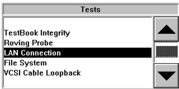
Touch the Integrity Tests button to view the Integrity Tests menu. Use the up and down arrows on the right - hand side of the scroll box to highlight your selection. Then touch Continue on the control panel to run the selected test. A new screen will appear and the test that you selected will begin automatically.
