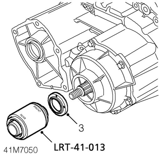
3. Using LRT-41-013 fit front output shaft oil seal to front casing. Ensure that seal is square to casing bore.
