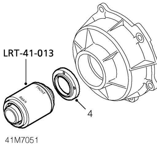
4. Using tool LRT-41-013 , drift oil seal into VCU housing. Ensure the seal is square to housing bore.
