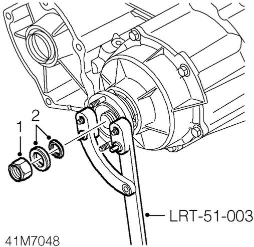
1. Using LRT-51-003 to restrain front output shaft drive flange, remove and discard nut securing drive flange to front output shaft.
