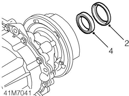
2. Remove dust shroud from transfer box rear casing.
