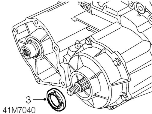
2. Using a flat bladed screwdriver free of rough edges, ease front output shaft oil seal from front casing.
