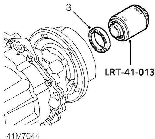
3. Using LRT-41-013 fit oil seal to transfer box rear casing.
