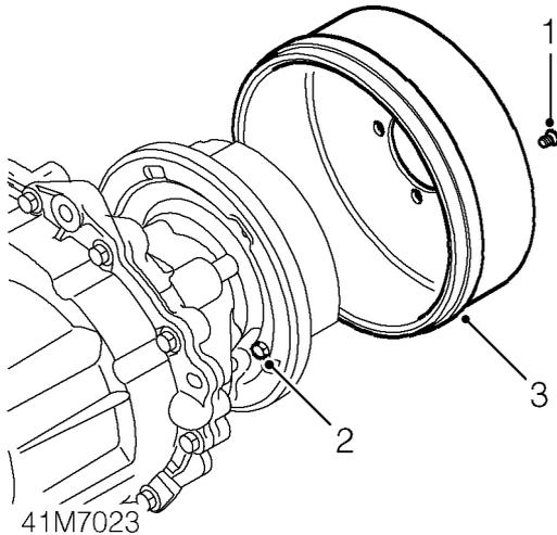
1. Remove screw securing brake drum to flange.
