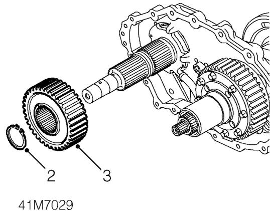
2. Remove circlip securing drive gear to intermediate shaft.
