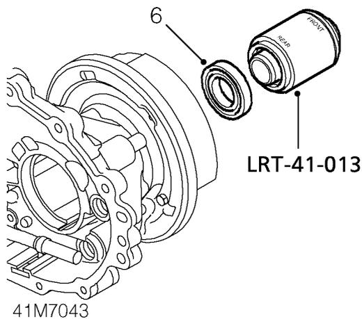
6. Using LRT-41-013, fit oil seal to transfer gearbox rear casing.
