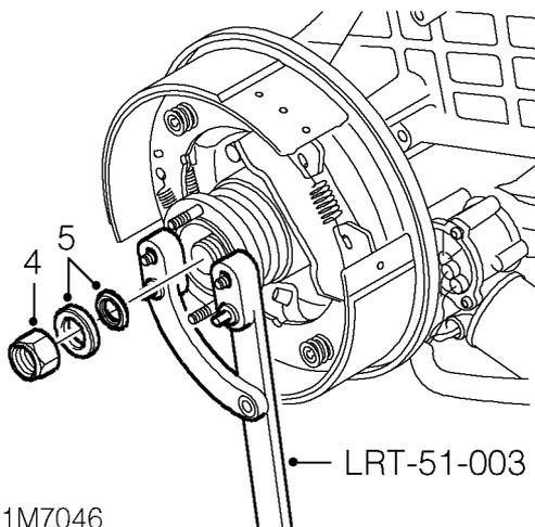
4. Using LRT-51-003 to restrain drive flange, remove nut securing drive flange to rear output shaft.
